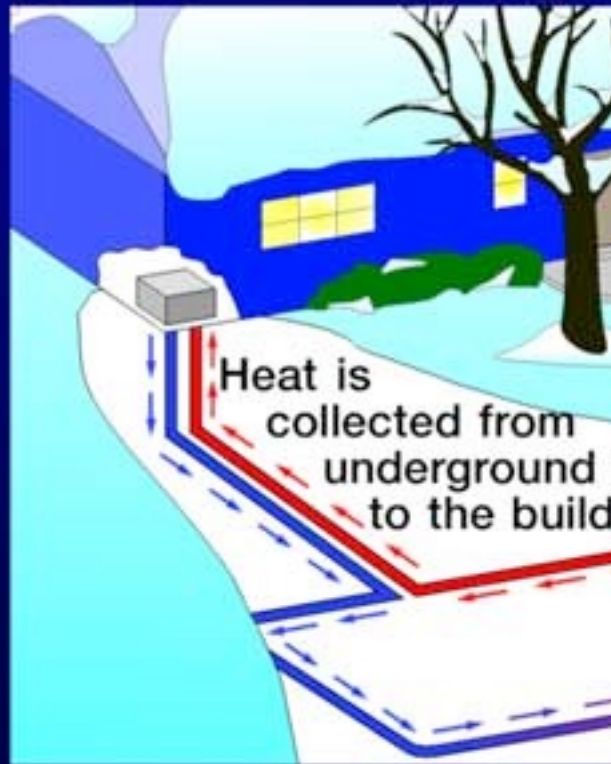
Heat Pump in Winter
